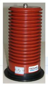
Techimp 1 nF Coupler is a capacitive coupler that applied for partial measurements. It can be chosen as PD sensor for Techimp PDCheck, PDScope or PDBasell systems. It is suitable for on/off line PD tests on rotating machines, for both spot measurements and monitoring applications, in fact it can be A BNC termination is permanently installed. available to connect the coupler through a coaxial cable. The 1 nF Coupler is fixed through 4 holes on the bottom flange.
